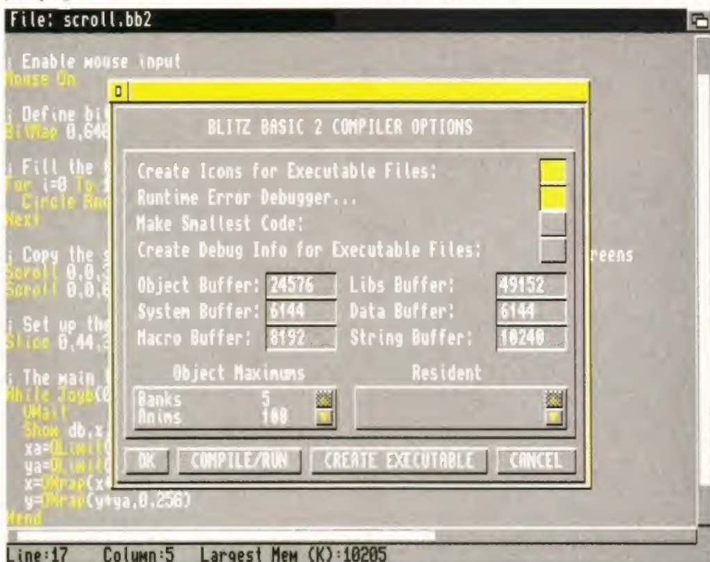
The Blitz Basic Compiler can be completely controlled without leaving the editor (TED), which all makes for a very easy-to-use programming environment. For example, you can get Blitz to compile all of your source code directly into stand-alone programs complete with icons.
